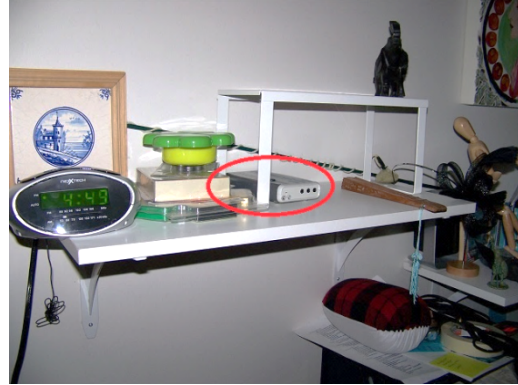
Figure 5: Datalogger measuring indoor air temperature and relative humidity.
