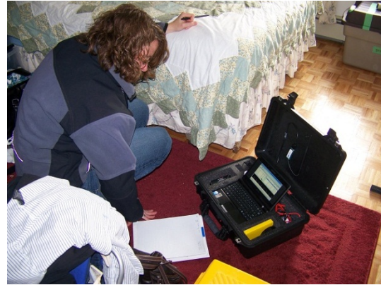
Figure 8: Wireless data download in progress from WiDAQ dataloggers to netbook.
