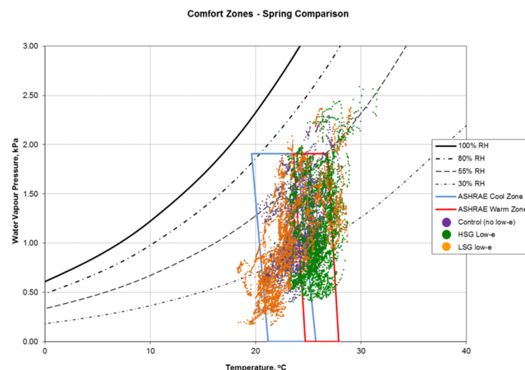
Figure 11: Measured indoor air temperature and relative humidity for all three study apartments, spring period.
