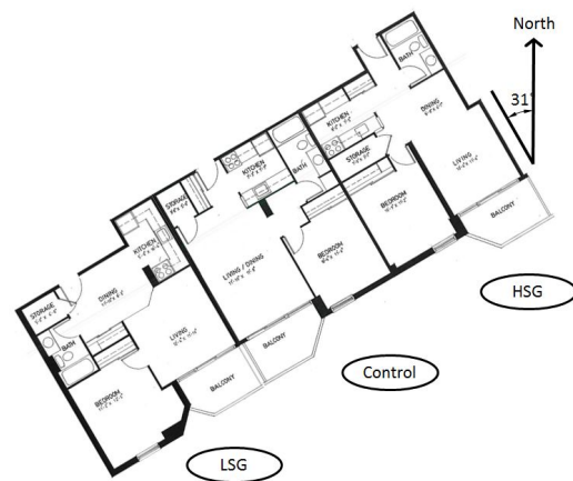
Figure 2: Floor plans of study apartments, oriented as in the building, facing east of south by 31°.
