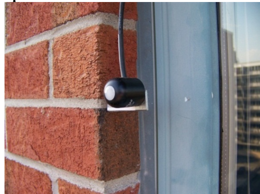
Figure 7: Pyranometer installed outside the HSG apartment bedroom window.
