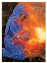
these locations, there is no class of PPE that can adequately protect the operator thereby precluding safe breaker operation or racking while energized. Even for less extreme approach boundaries, it is desirable to provide for remote operation accessories and procedures which place the operator outside of the potential hazard zone by providing a means to remotely operate and rack-out power circuit breakers while the switchboard is energized.
