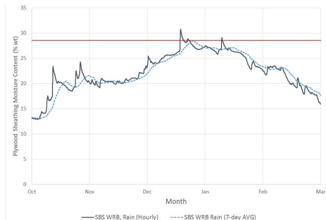
Figure 2: Comparison of hourly and 7-day running average plywood sheathing moisture content of east-facing split insulated wood-frame wall in Vancouver with 1% rain penetration, not subjected to air leakage.
