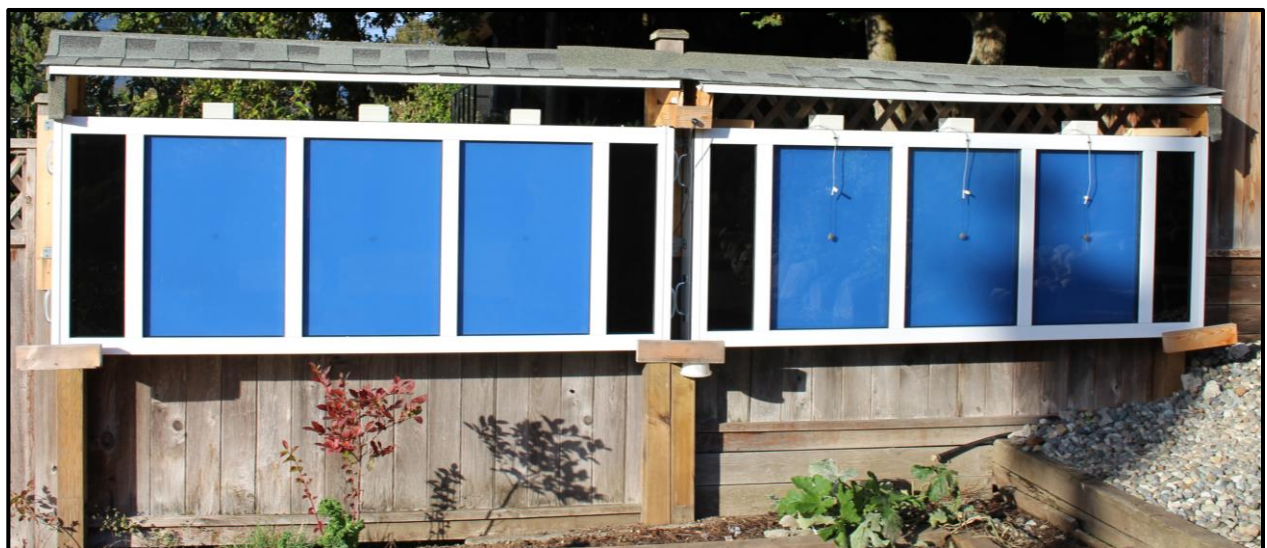
Figure 4: Installed Mockup with Opacified Glass Installed
