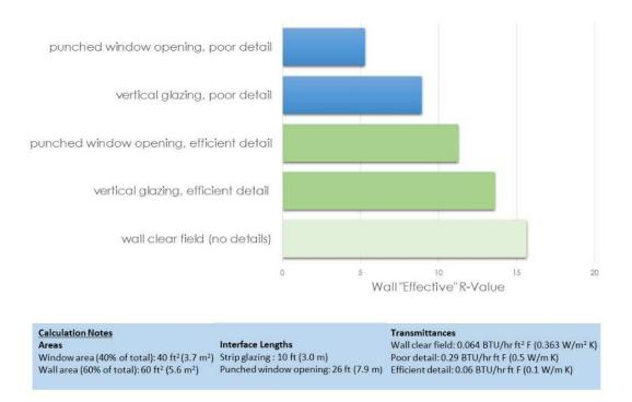
Figure 1: Impact of the Window to Wall Interface
