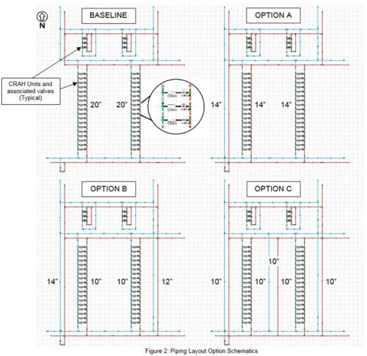
Using the modeling software to calculate system flowrate and head, the chilled water piping sizes are optimized under each configuration. Each option represents an effective piping scheme, and is acceptable based on project requirements. Adding the extra piping runs decreases the necessary size of other pipes within the system, representing a tradeoff between size and quantity of piping and the overall capital cost.
