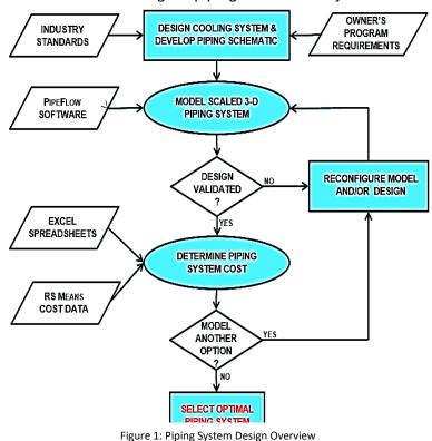
can be exported to Excel for further analysis and customized spreadsheets can then be used to compile the total length of piping, the total number of valves, and the total number of fittings. All of these are classified by pipe diameter, from which RS Means cost data is used to determine the total installation cost of the modeled system. The model and cost data are then archived and alternate piping configurations are analyzed for comparative purposes.
