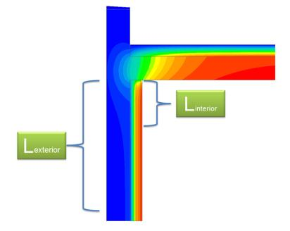
FIGURE 1: Effective lengths for parapet from exterior and interior
